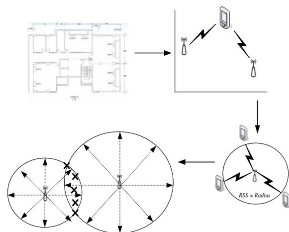
Fig. 3. Position determination overview
