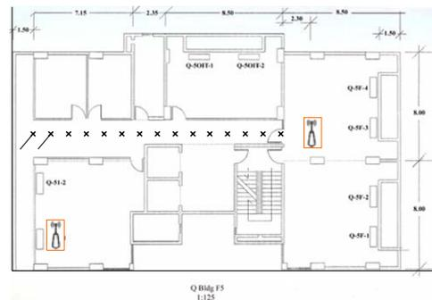
Fig. 1. Q5 floor plan with markers and access points locations
